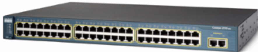
Figure 4 Cisco Catalyst 2950T-48 Switch
